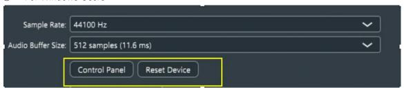
When using ASIO driver, you can use control panel of the Audio Interface.
