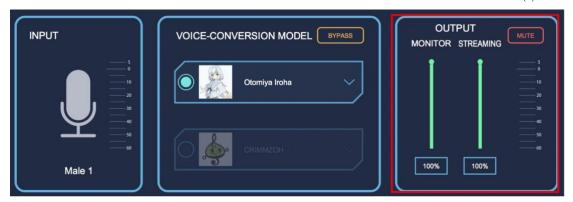
To avoid sound clipping, please adjust your voice while checking the OUTPUT level meter. In addition, you can mute the output audio by clicking "Mute" or pressing Enter key. (While it's working, the button turns red.)
