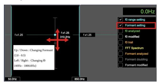
By moving the light blue point in the direction of the crossed arrows above, you can set the Formant and Formant Center values. You can also change the formant slope by dragging the thin light blue line. VUV
