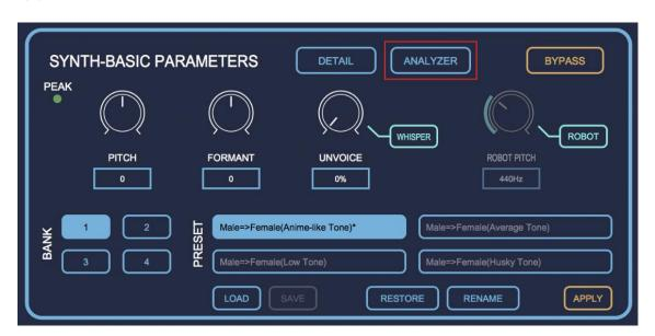
By clicking "ANALYZER" on the main screen of Voidol SYNTH, you can see the analyzing screen for the audio information processed by Voidol SYNTH. In the ANALYZER screen, you can monitor each parameter of audio information and also can set parameters such as f0 (detected speaker's pitch) and formant.
