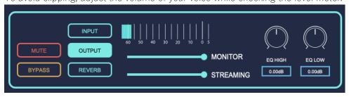
The STREAMING parameter sets the volume sent to the virtual driver "Voidol Audio". (\*) Audio can be sent to capture software such as web conferencing systems and OBS. The virtual driver "Voidol Audio" is included only with the Windows version. (Automatic installation) The macOS version requires a separate virtual driver from another company, such as VB-CABLE. In the macOS version, the OUTPUT meter does not work unless the Streaming Device is set.
