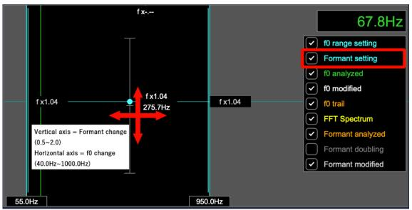
By moving the light blue point in the direction of the crossed arrows above, you can set the Formant and Formant Center values. You can also change the formant slope by dragging the thin light blue line.
