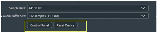
When using ASIO driver, you can use control panel of the Audio Interface.
