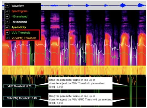
For VUV Threshold and VUV(PM) Threshold, you can set the parameters by dragging up/down the parameter name or line displayed on the ANALYZER.
