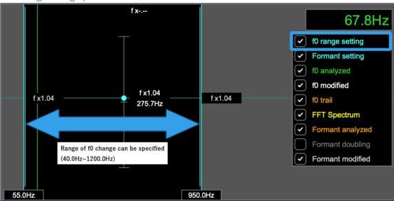
By moving the light blue bars on the left and right of the above image arrows, you can adjust the range of the f0 change. By keeping the lowest and highest tones of the speaker within the range, good quality conversion is possible.
