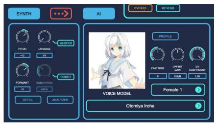
\* In the image above, SYNTH > Al conversion is selected, and the given SYNTH configuration increases the pitch of the voice to make it more feminine, then it is converted using the Female 1 model of "Otomiya Iroha".
